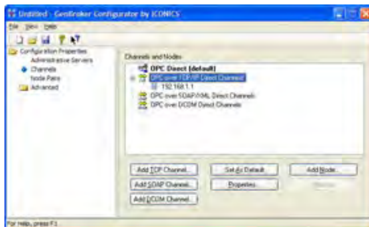
Figure L8.6: GenBroker Configuration for the Client (Mywebserver)
