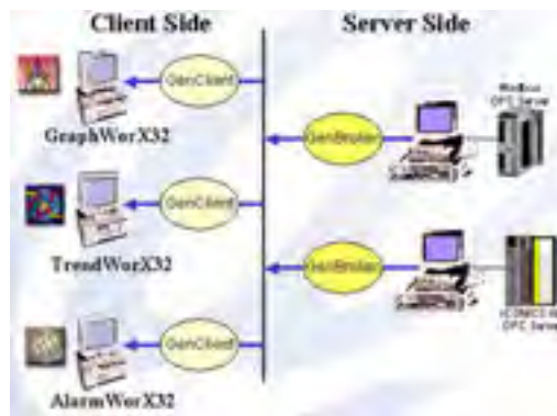
Figure 3.4: OPC Direct Channel Over DCOM (Intranet Only)
