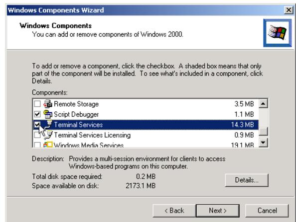
**Figure 2 - Installing Windows Terminal Services**
