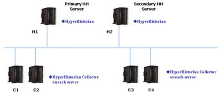
Figure 2 - Example Scenario of Hyper Historian Redundancy
