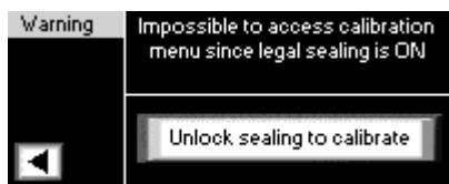
You must confirm to unlock legal sealing if you want to access to calibration. If so, a new legal CRC will be calculated and legal counter incremented
