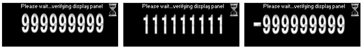
When the legal for trade mode is active, the display is checked at each power-up or connection
