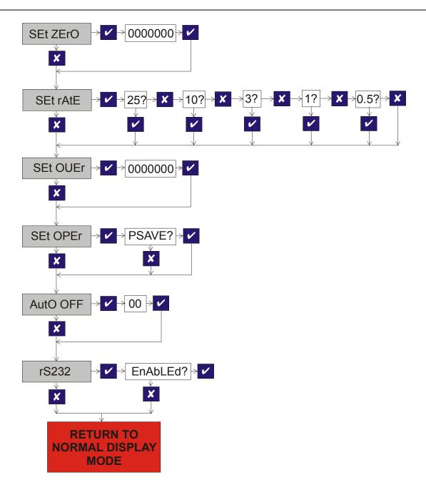
A Calibration Menu, which is used to calibrate each of the two ranges with independent scales, as well as setting the display resolution for each range.
