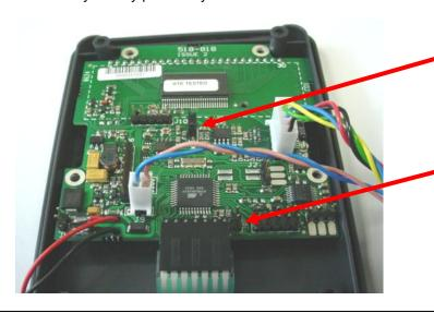
Sensitivity link should be in this position for use with sensors, with sensitivities <+/- 5mV/V
