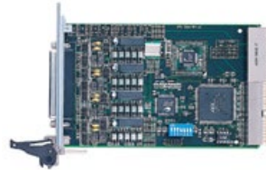
cPCI-3544: 4-Port RS-422/485 Isolated Serial Communications Card
