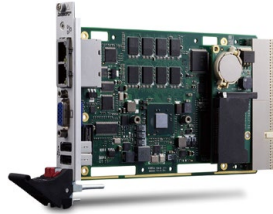
cPCI-3615: 3U CompactPCI® Dual-Core Intel® Atom™ Processor Blade
