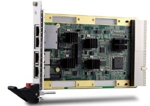
cPCI-3E10: 3U CompactPCI® 2/4-Port Gigabit Ethernet Card
