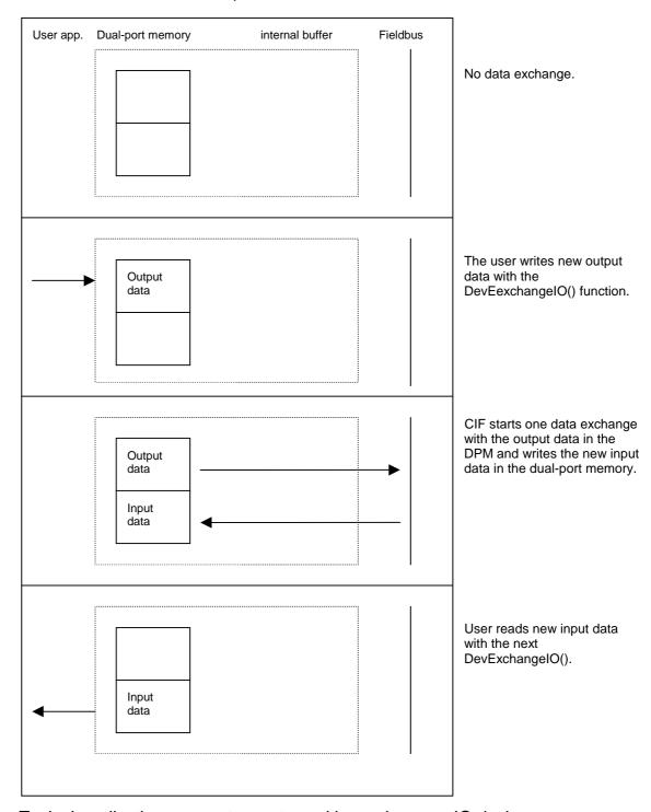
Typical application: master system with synchronous IO devices.
