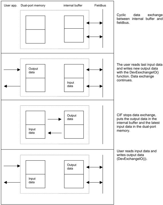
Typical application: easiest handshake in master and slave systems with a guaranteed consistence of the complete process image.
