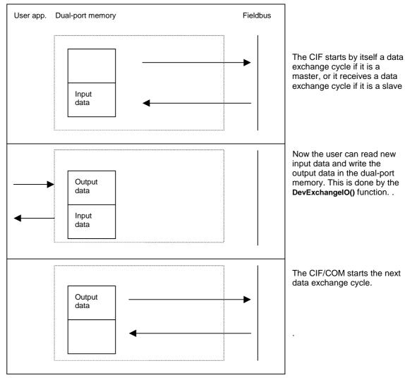
Typical application: slave system, which must guarantee that the data from every master cycle must be given to the user program.
