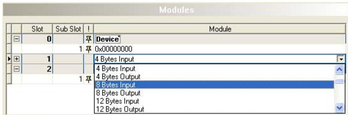
Figure 11: Changing Modules using Drop-Down Control (\* The Name of the device is displayed.)
