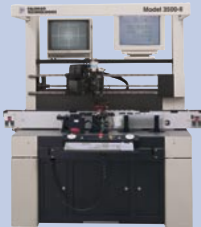
Figure 14: Palomar 3500 automatic die attach
