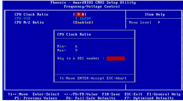
The CPU clock ratio is set by the BIOS, depending on the processor version used. Usually, this is the best setting possible. Changing these values is only recommended for very experienced users and should only be attempted after studying the processor's datasheet.
