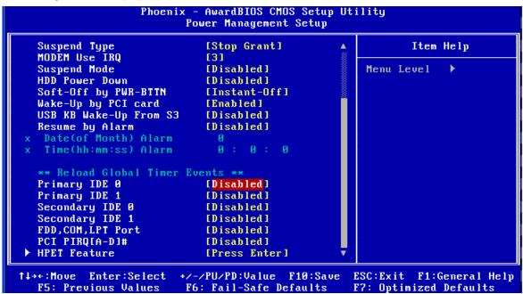
When enabled, the Reload Global Timer Events allow restarting the global standby timer when such an event occurs.
