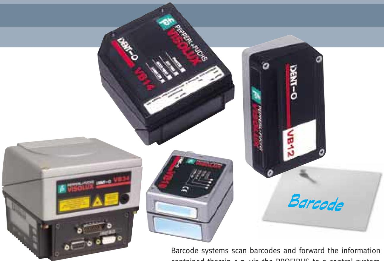
Barcode systems scan barcodes and forward the information contained therein e.g. via the PROFIBUS to a control system. Scanning takes place according to the reflection principle by means of ruby light.
