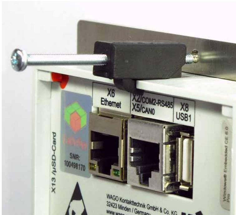
Figure 9: Detailed photograph of installation with intermediate plate
