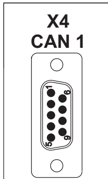
Figure 6: Connector X4 – CAN 1 interface D-Sub 9
