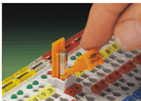
Fig. 2-16: Opening the fuse carrier
