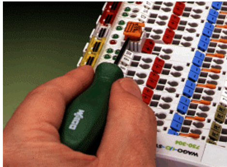
Fig. 2-15: Removing the fuse carrier
