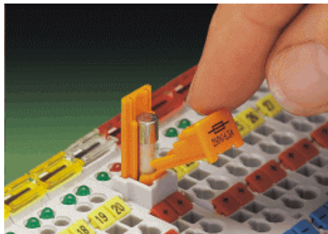
Fig. 2-16: Opening the fuse carrier
