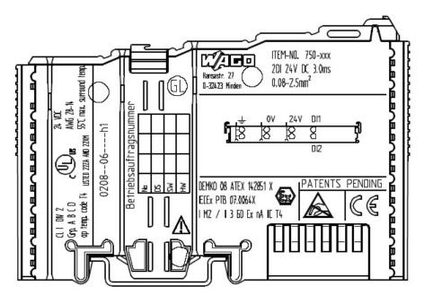
Figure 12: Side marking example for ATEX and IEC Ex approved I/O modules according to CENELEC and IEC
