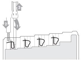
Figure 11: Connecting a conductor to a CAGE CLAMP®
