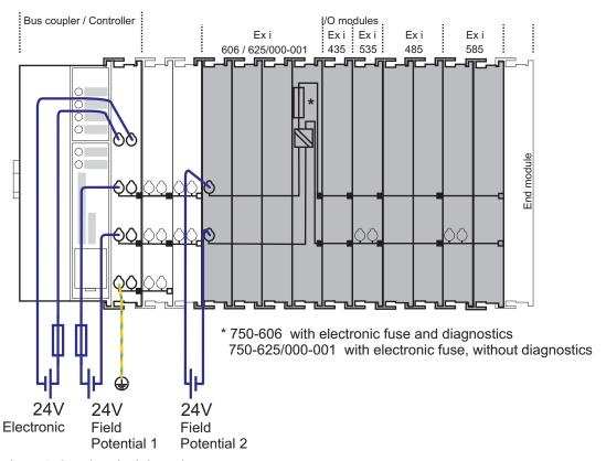
Figure 1: Supply Principle Ex i
