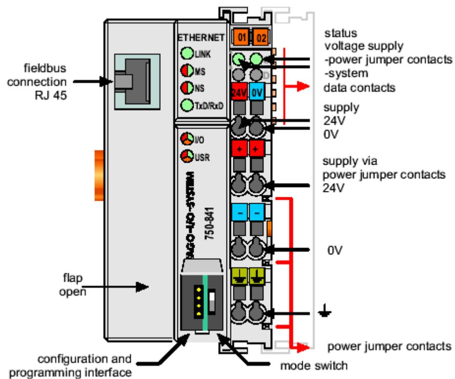
Fig.1: 10/100 MBit ETHERNET fieldbus controller 750-841
