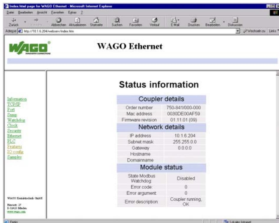
The screenshot shows the WAGO Ethernet Web Management Interface (WBM) home page. The page is titled "WAGO Ethernet" and features a navigation menu on the left with links for Information, TCP/IP, Port, Smpg, Watchdog, Clock, Security, Ethernet, PLC, Features, IO config, and Sampler. The main content area displays "Status information" with three sections:
