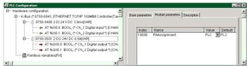
Fig. 14: WAGO-I/O-PRO CAA, PLC configuration with 750-400 and -501
