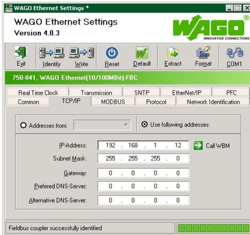
Fig. 4: Settings of the 750-841 Controller IP address
