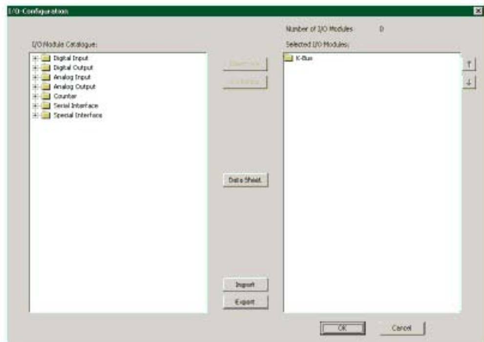
Fig. 13: WAGO-I/O-PRO CAA, with I/O configuration dialog
