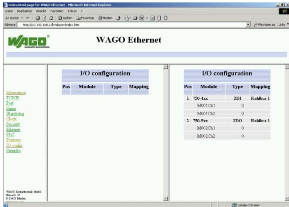
Fig. 8: “IO config“ page of the integrated WEB server
