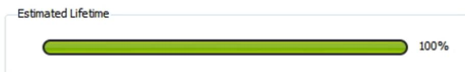
**Note:** The formula for calculating estimated lifetime is: Current Avg. Erase Count / MLC guaranteed P/E cycle x 100%
