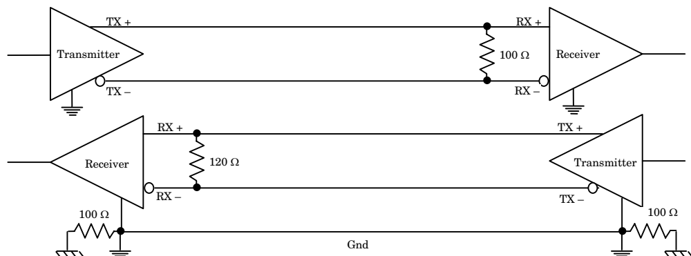
Figure 5-4 Typical RS-422 four-wire interface circuit
