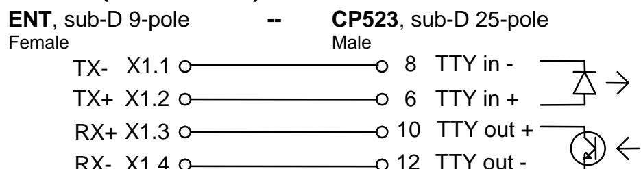
**Note:** The jumpers for the 20 mA interface in the ENT-DC must be set to "active, active" (see ENT-DC Technical Manual).
