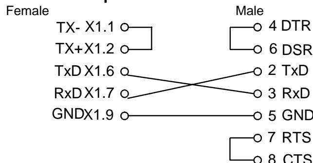
**Note:** The Tx jumpers for the 20 mA interface in the ENT-DC-1 must be set to "active". The Rx jumper setting is not relevant (see ENT-DC Technical Manual).
