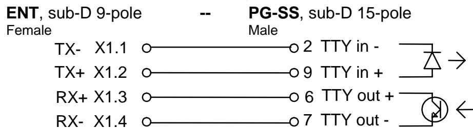
**Note:** The jumpers for the 20 mA interface in the ENT-DC must be set to "active, active" (see ENT-DC Technical Manual).
