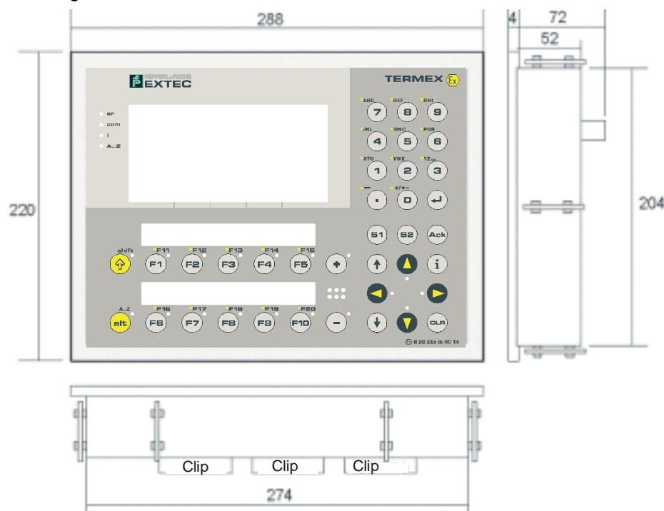
Fastened with 6 clamping mounting plates (included in the scope of supply)
