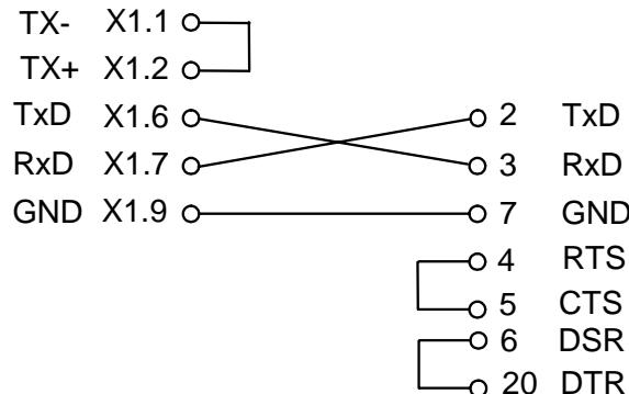
**Note:** The Tx jumpers for the 20 mA interface in the ENT-DC-1 must be set to "active". The Rx jumper setting is not relevant (see ENT-DC Technical Manual).
